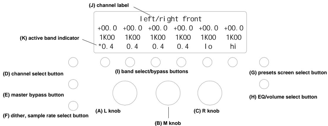
Figure 1 - z-Q6 front panel controls
